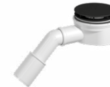
Shower tray siphon, drain hole Ø90mm, low version, drain pipe 40/50mm, ABS knob, black matt
