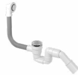
Bathtub siphon with overflow, cleaned from above, stainless steel click-clack plug Ø 70mm, drain pipe 40/50mm
